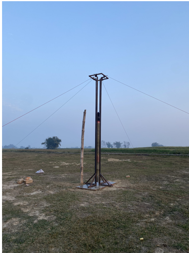
Figure 4.21: Rocket body loaded in Launch Stand
