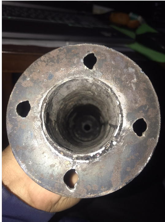
Figure 4.6: Stainless Steel Tube as Combustion Chamber
