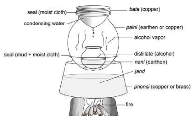
Figure 1.2: Traditional raksi distillation setup (Adapted from [7])
